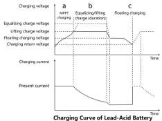
The charging stages of lead-acid batteries include MPPT charging, constant voltage charging (equalizing/lifting/floating charging) and current limiting charging.
