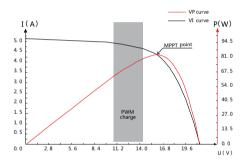
Fig.1-2 Output Characteristic Curve for Solar Battery
