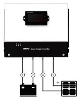
Warning: : Danger of electric shock! We strongly recommend to connect the fuse or breaker at the photoyoltaic array and the battery terminals to prevent electric shock hazard in wiring or inaccurate operation. Furthermore, before wiring, it is required to guarantee that the fuse or breaker is in open state.
