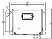
Product size : 314\*259\*121mm Installation size : 228\*171mm Fixing hole position : Φ8mm Wire specification : 20-2AWG
